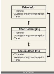
To change the trip mode, toggle the switch (//) on the steering wheel.
