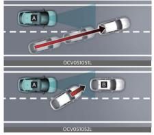
[A]: Your vehicle, [B]: Front vehicle If a vehicle cuts in front of your vehicle, Leading Departure Alert may not operate properly. • When the vehicle ahead sharply steers
