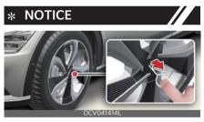
For 20 inch wheel, take out the remover tool in the Tire Mobility Kit. Insert the tool to the hole and pull out the wheel cover.
