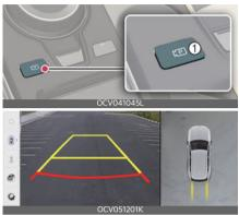
Surround View Monitor can assist in parking by allowing the driver to see around the vehicle.
