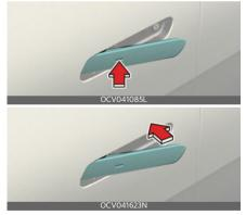
When all doors are closed, touch the touch sensor on the front outside door handle (the engraved part) while carry<sup>-</sup> ing the smart key with you, outside door handle will return and doors will be locked.
