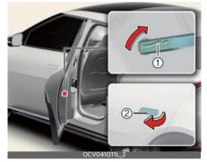
To lock the child safety lock, insert a key (or screwdriver) into the hole and turn it to the lock position.
