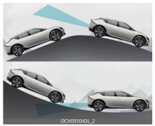
Blind-Spot Collision-Avoidance Assist may not operate properly when driv<sup>-</sup> ing on a sloped road. Blind-Spot Collision-Avoidance Assist may not detect the vehicle in the next lane or may incorrectly detect the ground or structure.
