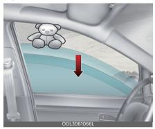
If the window detects the resistance while the power window switch is pulled up continuously, the window will stop upward movement then lower approximately 1 inch (2.5 cm).
