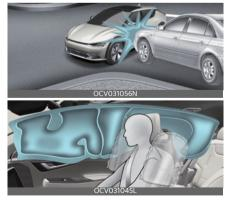
Side and/or curtain air bags are designed to inflate when an impact is detected by side collision sensors
