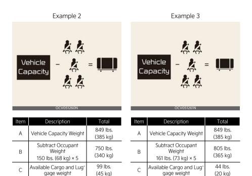
Refer to your vehicle's tire and loading information label for specific information about your vehicle's capacity weight and seating positions. The combined weight of the driver, passengers and cargo should never exceed your vehicle's capacity weight.
