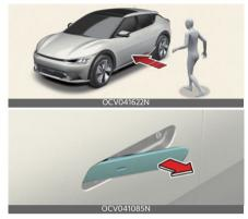
If you approach (within 1 ft. (30 cm)) the driver or front passenger's door handle possessing the smart key, the outside door handles slide out and the doors are unlocked. In this case, Hazard Warning Flasher blinks twice and chime also sounds twice.
