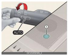
When the light switch is in the AUTO light position, the taillights and head-lights will turn ON or OFF automatically depending on the amount of light outside the vehicle.
